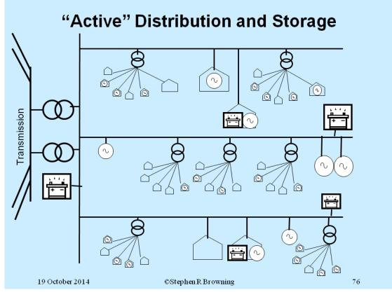
A lot of individual data is required for distribution system (microgrid) security management, and the aggregated information by supply point is then required by the market and the system operator for demand-generation matching and to maintain transmission integrity.
