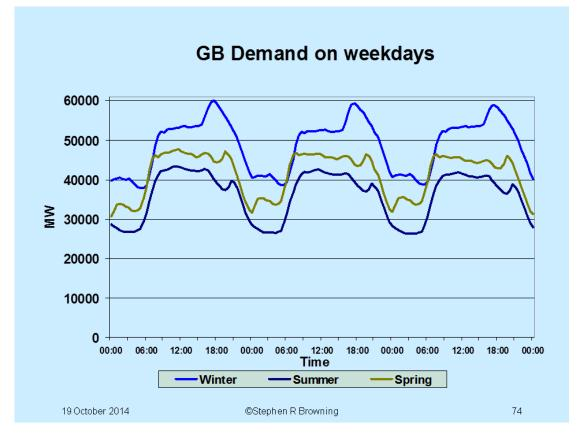
The objective is to both reduce and smooth the power output of fossil fired generation while making the residual requirement for such plant predictable. This will not only reduce the energy requirement, but also, when such a plant is required, ensure it runs at peak efficiency to avoid unnecessary fuel burn and emissions.
